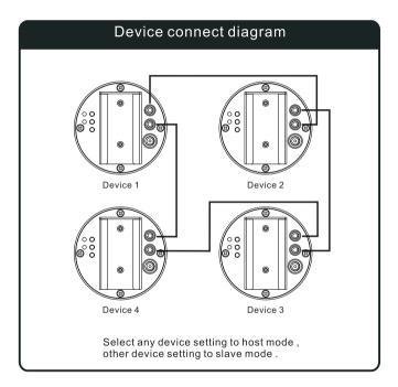
If there are more devices, the link way is the same. When multiple devices linked, only one device is in master mode, and other devices are in slave mode. Devices that have been linked to the network will maintain their own master-slave mode. If the power is turned off, the settings will not be changed.
