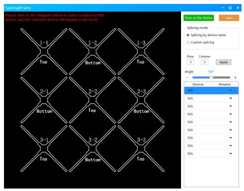
D. The Device Name Splice Mode is more commonly used. The Custom Splice Mode is only used for irregularly shaped displays or professional usage.
