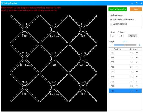
H. To adjust the device angle, click on the device, and adjust the number for "device angle".
