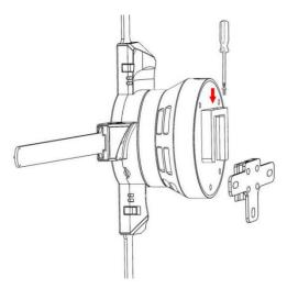
D. Install all the devices according to the instructions above. Manually spin the fans at a low speed to ensure the light bars will not hit each other. After the padding is installed, the distance between light bars on neighboring devices must be greater than 1 cm to be safe. After you finish the check, you can turn on the power to test them.
