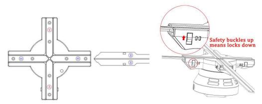
C. Mount the device on the base and fix the safety screw according to the following diagram:
