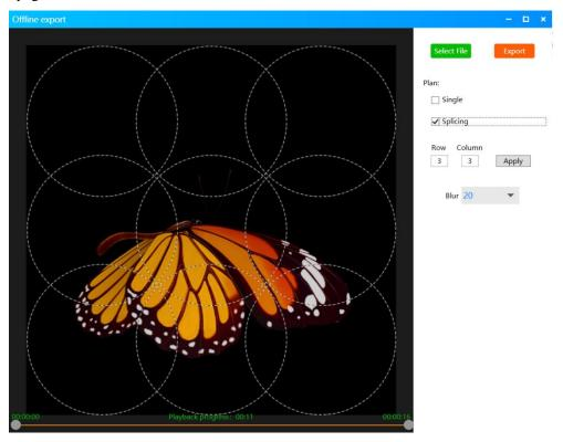
There are two modes for offline export: Standalone Mode and Splice Mode. In Splice Mode, you need to configure the number of rows and columns and click "apply". The device schematic diagram will change accordingly. Then, click "select file", adjust the file content, and click "export". And select a folder to save the files. The export files will be named as device position + file name. For example, "1-1\_butterfly.ftlv" represents the edited file for the
